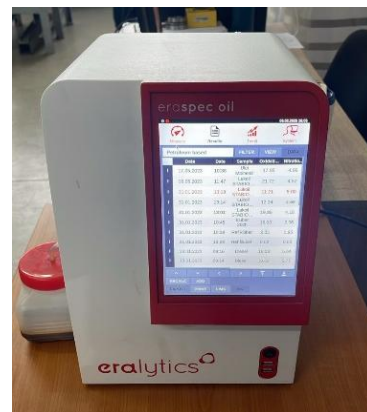
Fig. 2.4 Lubricant Analysis - Portable equipment for oil analysis
