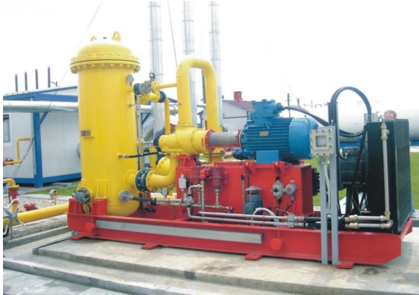
Fig. 1.1 Electrocompressor Installed in a Gas Extraction Park
