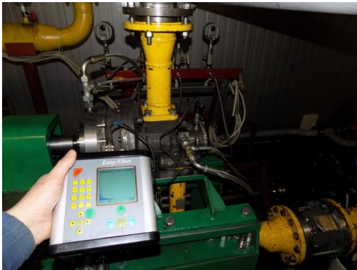
Fig. 2.1 Vibration Level Analysis - Viber X1 vibration analyzer measuring the compressor's vibration level
