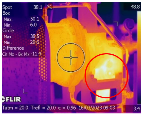
Fig. 3.3 Thermographic Analysis of the Compression Unit
