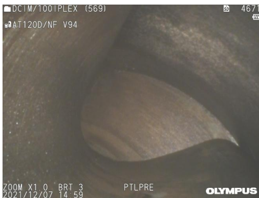
Fig. 2.3 Borescope Analysis - Internal visualization of the condition of the screw rotors
